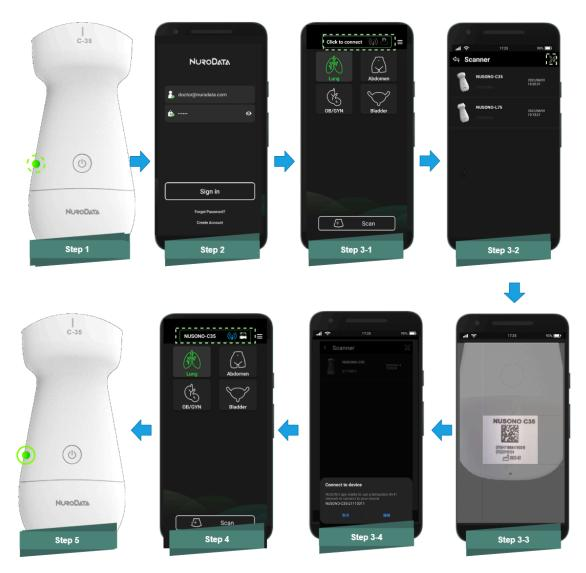
ultrasound device from the charging dock and start the first device connection setup operation.
