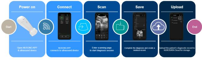
You can operate the ultrasound device through Wi-Fi Direct.
